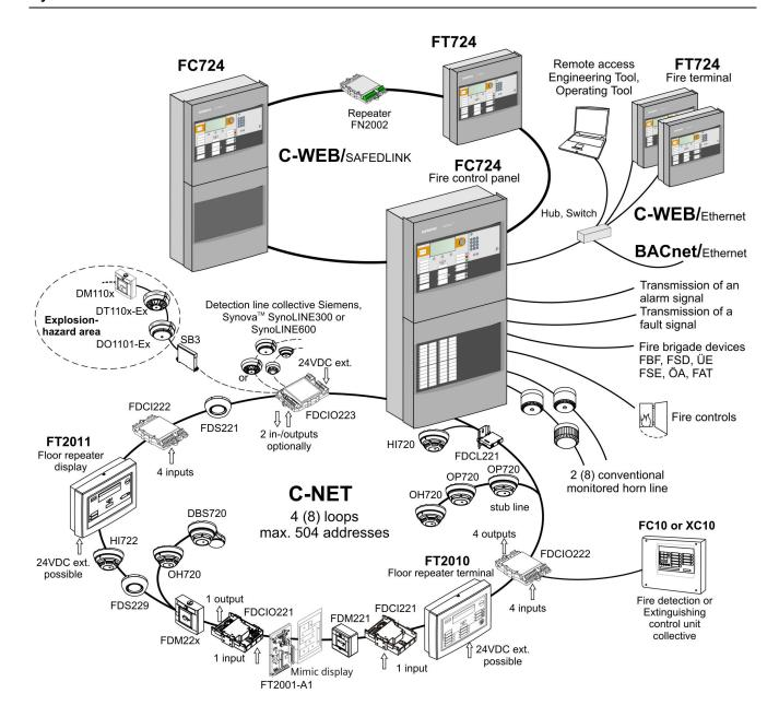
The high-performance C-WEB makes it possible to network up to 16 FC724/722 fire control panels and FT724 fire terminals together as required. The innovative redundant network nodes not only set new standards in terms of failsafe characteristics but also for high-speed data transfer.
